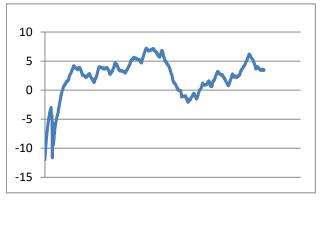
the standard NTP protocol to get time from a Velasync time server. Error is well below 100 microseconds with no special network cards, protocols or switches.
