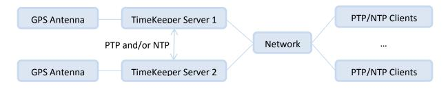
If a direct GPS signal is not an option, CDMA can provide a reasonably accurate time source. If neither GPS or CDMA are available, the server can consume existing NTP and PTP on the network, and deliver that to downstream clients. This is a stratum server (in NTP terminology) or boundary clock (in PTP terminology), and can be used as a means to deliver a reliable time signal from deeper in the network than a single top level server.
