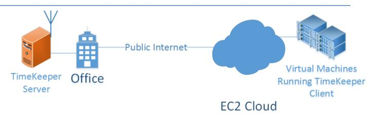
The clocks on Cloud Virtual Machines are notoriously inaccurate and hard to synchronize with legacy technology but can be tightly controlled using TimeKeeper. One simple method is synchronize TimeKeeper enabled cloud VMs to an external TimeKeeper reference. Our tests show that clocks remain within 15-25 microseconds of reference in such a setup even with standard Internet access. The result is to make practical, high precision time accuracy a low cost, trivial to implement, utility on the Cloud.
