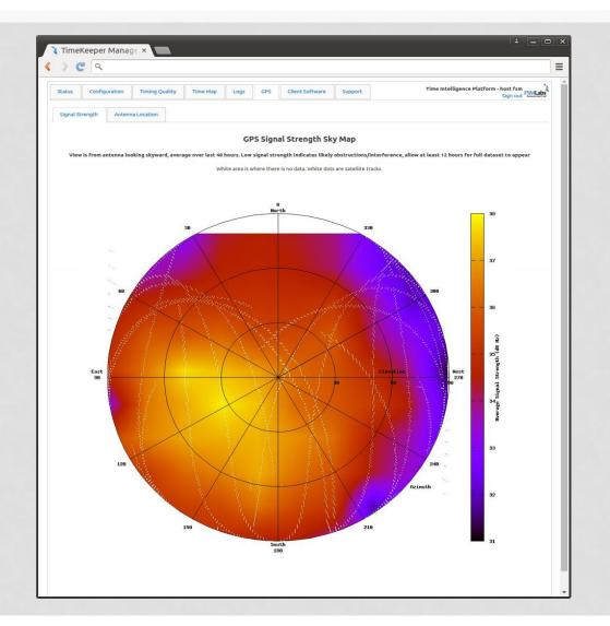
Build specialized heat map from GPS signal data so show composite picture of signal strength. Purple areas show blocked reception.
