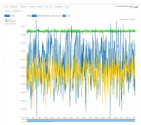
This is not a short burst of accurate time either - it's a full 24 hour period of testing where time went from GPS via NTP/PTP to Windows and back all without deviating by more than a single microsecond.
