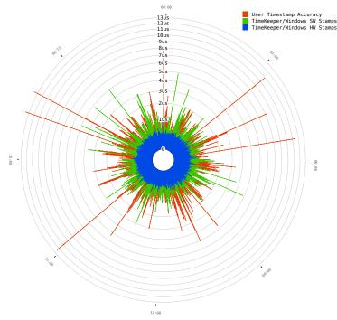
Zeroing in - 24 Hours of TimeKeeper/Windows Accuracy with Hardware Timestamping
