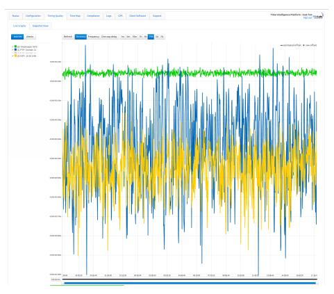
This is not a short burst of accurate time either - it's a full 24 hour period of testing where time went from GPS via NTP/PTP to Windows and back all without deviating by more than a single microsecond.
